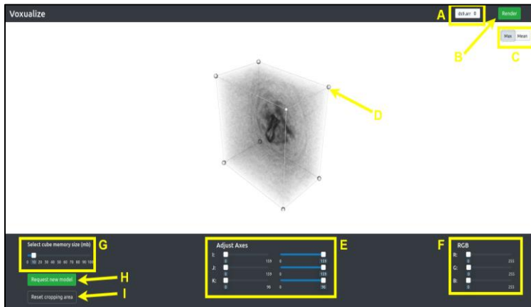
Figure 5: The UI of Voxualize. This screenshot was taken just after a file was selected and the “Render” button pressed.
